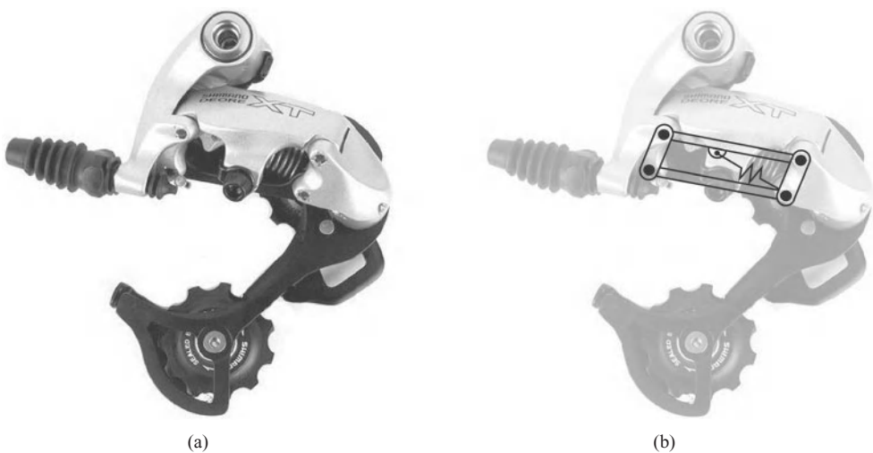
Figure 8.8 (a) Shimano Deore XT (rigid-body mechanism), and (b) Simplified sketch of the mechanism
