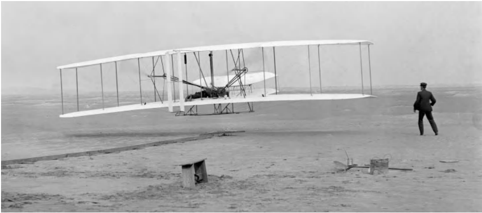
Figure 1.3 The Wright brothers used wing warping to achieve control of their aircraft for sustained human flight
