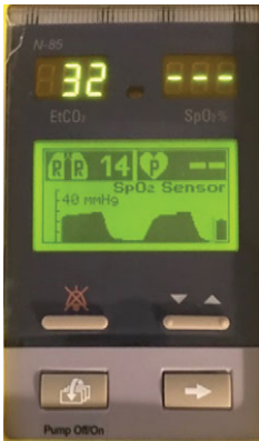
Figure 2.6 Hand held capnography device showing a good CO 2 waveform (Photo: Colin Kaide)
